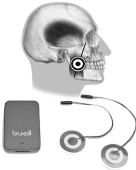
Fig. 1. The Bruxoff ®* and the CoDe ®* electrode used in this study for the detection of myoelectric signals from the masseter muscles. This electrode was chosen to avoid any orientation problem. At the top, a schematic representation of the electrode location over the masseter muscle is shown. Black line: gonial angle-cantus line used as anatomical landmark.
