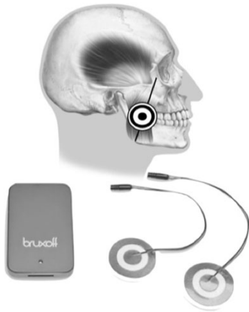
Fig. 1 The Bruxoff ® and the CoDe ® (Spes Medica, Genova, Italy) electrode used in this study for the detection of myoelectric signals from the masseter muscles. The concentric-ring systems of the Code electrodes show higher spatial selectivity with respect to the traditional detection systems and reduce the problem of electrode location since they are invariant to rotations and reducing EMG cross talk. At the top, a schematic representation of the electrode location over the masseter muscle is shown. Black line gonial angle-cantus line used as anatomical landmark
